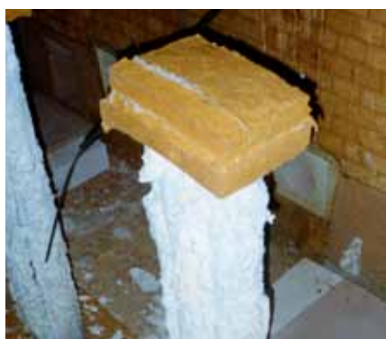
Brandwerende coating na verhitting
